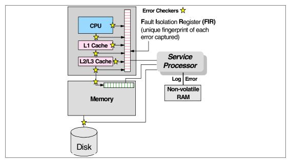
Figure 3-2 Fault Isolation Register
