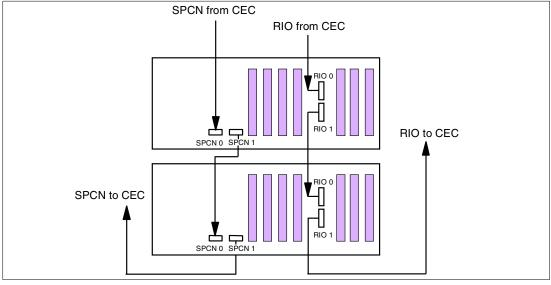
Figure 2-7 Remote I/O and SPCN cabling
