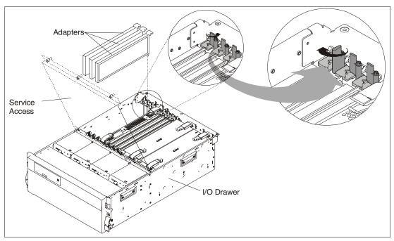
Figure 2-5 Inside view of 7311-D20 I/O drawer
