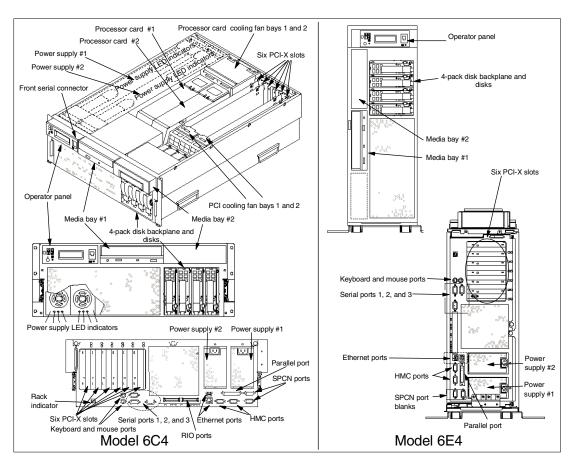
Figure 1-1 Views of Models 6C4 and 6E4 (POWER4+ system with six PCI-X slots)
