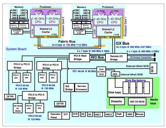
Figure 2-1 Conceptual diagram of the Models 6C4 and 6E4 POWER4+ system architecture
