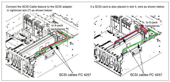
Figure 2-8 Internal SCSI cabling
