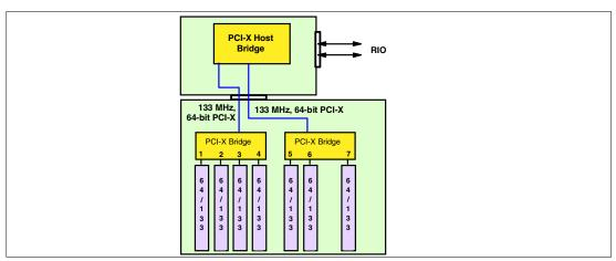
Figure 2-6 Conceptual diagram of the I/O drawer
