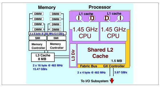
Figure 2-4 Conceptual diagram of POWER4+ processor and memory subsystem
