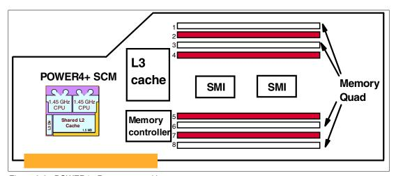
Figure 2-3 POWER4+ Processor card layout
