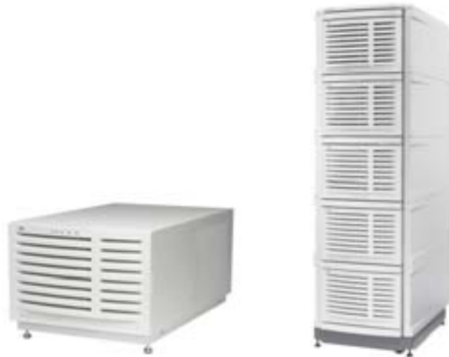
figure 3. the hp server rx5670 is suitable for rack-mount or standalone duty
